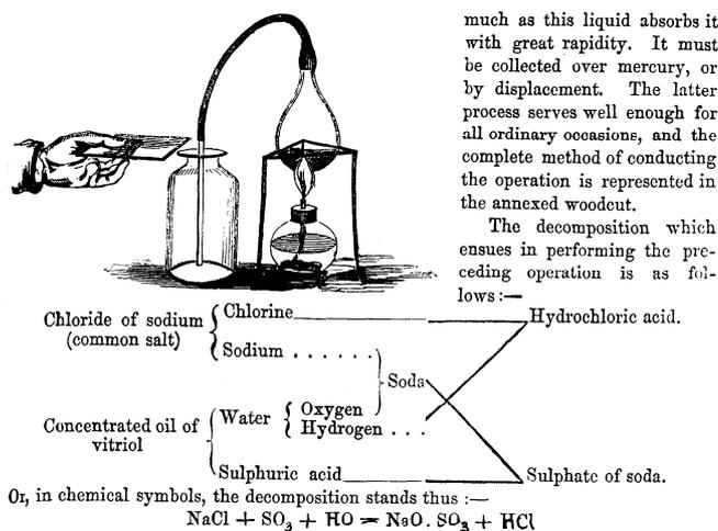
Figure 7: Three ways of depicting the preparation of hydrogen chloride from common salt (from Scoffern 1852, p. 357).
