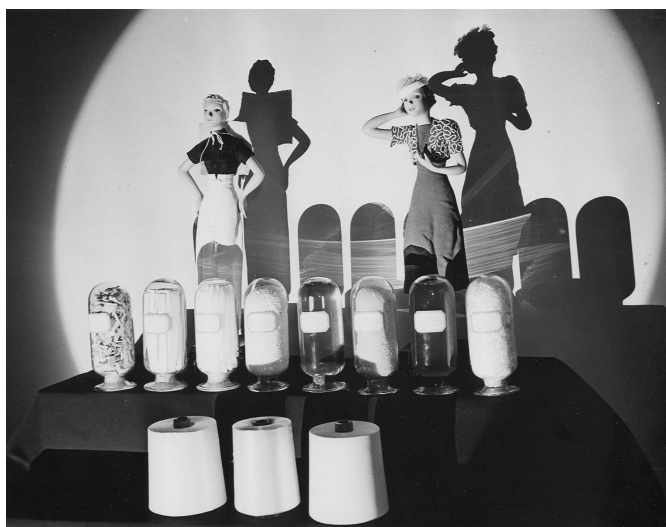
Figure 3. Steps in making rayon, a photograph by Fremont Davis which was supplied with the Science Service ‘Fabrics for the Future’ newspaper series, 1939. The suggested caption read “Eight different chemical steps go into the making of acetate rayon in turning raw wood chips into the finest of fibers and fabrics.” (SIA RU7091, Box 408, Folder 23). Courtesy of Smithsonian Institution Archives.
